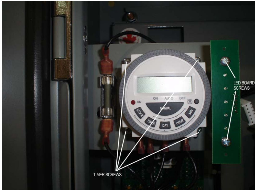
Figure 8. TIMER AND LED BOARD SCREWS
